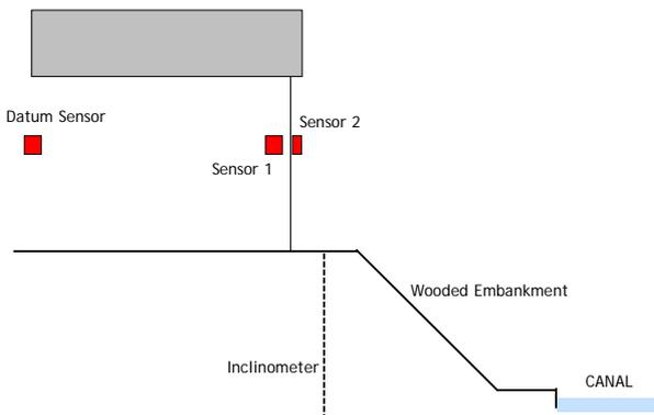
There is a question mark over the cause of movement to this two storey structure which has been built very close to a steep slope in the Mercia Mudstone.
